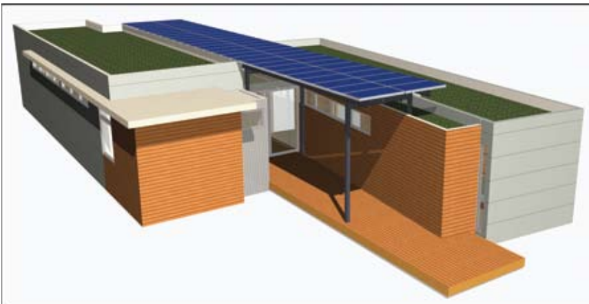
The Solar Passage fits on a 50' lot and it looks inward on the lot. It's also designed to provide as much light in as possible. It has a solar orientation with cross-ventilation. The model runs 1,540 sq. ft. in a three-bedroom plan with decks, green roof and a solar panel covered entry.
